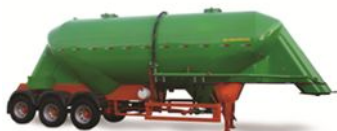
Cement Bulk Trailer
